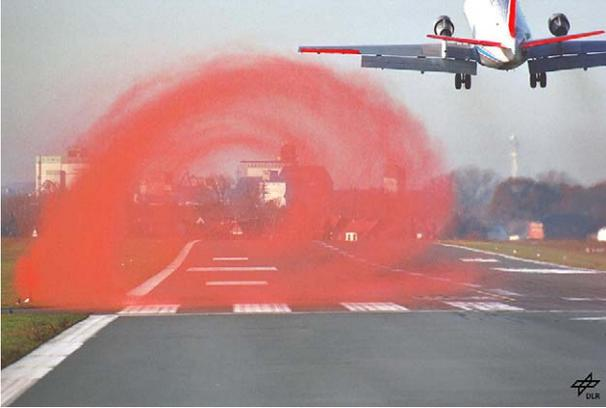
Fig. 1. DLR test aircraft ATTAS with visualised wake vortex.
